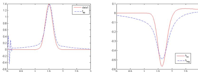
FIGURE 2. Test 1 (Method 1): (left) exact and approximate solution at  $x = 0$ ; (right) exact and approximate heat flow at  $x = 1$ , with  $\delta = 0$ ,  $M = 80$ .
