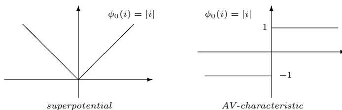
FIGURE 2. Diode Model
