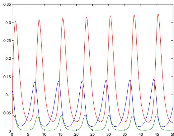
FIGURE 3. Oscillatory behavior for the system studied in this section. The parameter values are  $x_0 = .05$ ,  $c_2 = 5$ ,  $c_3 = 1.2$ , and  $c_4 = 99$  (so  $c_1 = 1$ ). The critical value is  $c_4^* = 95.4$ . In the graph, the values of  $z(t)$  (red) are divided by 10 to make the scaling compatible
