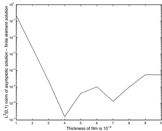
**Figure 1:** Comparison of asymptotic and finite element solutions: The pump (fundamental) fields.
